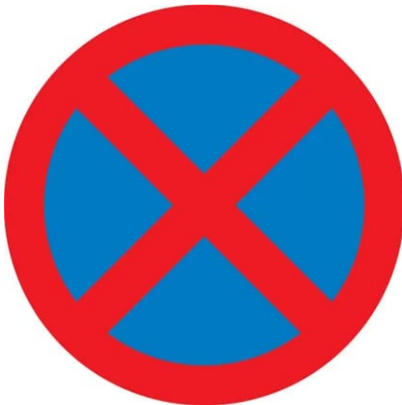
No stopping (Clearway)
