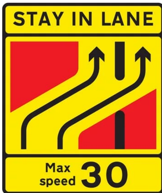
One lane crossover at contraflow road works
